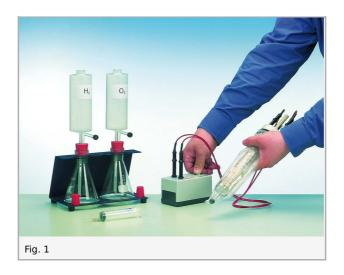
After having checked if the explosion eudiometer is in a flawless condition according to its operating instructions, connect the two electrical contacts to the ignition spark generator (Fig. 2).
